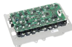
Fig. 2: Newly developed intelligent power module
