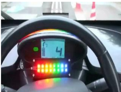
Figure19: Photograph of an LED panel while the EV was running on the test road
