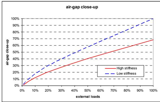
Figure16: In-Wheel motor air-gap close-up
