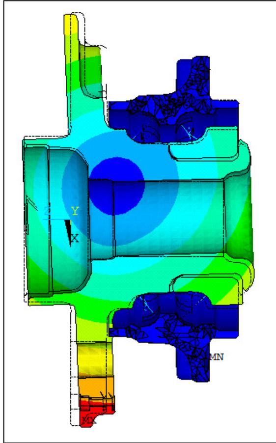
Figure14: bearing flange deflection under extreme cornering external loads
