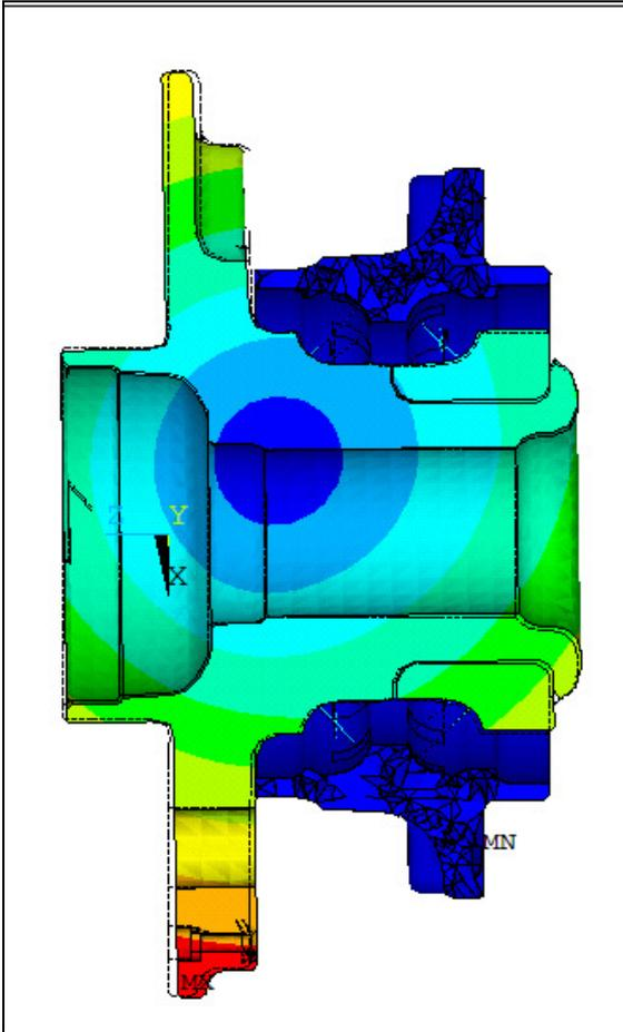
Figure13: bearing flange deflection under low cornering external loads
