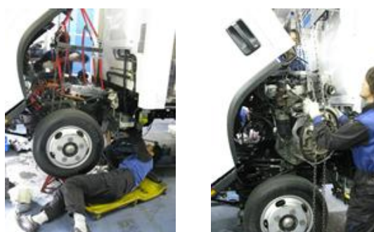
Figure 6: Conversion at Local Body Shop (engine dismantling and motor unit instalment)
